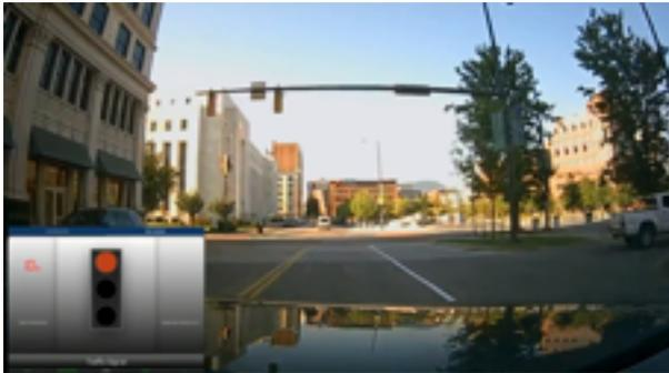
Researchers at CUIP are studying implementations of real-time data from SPaT (signal phase and timing) and the benefits of that data being transmitted from signalized intersections to vehicles via DSRC (dedicated short-range communication). Large scale deployment of this technology would make for significantly safer streets through signal violation warnings, traffic signal adaptations, pedestrian and biker alerts at intersections, and
