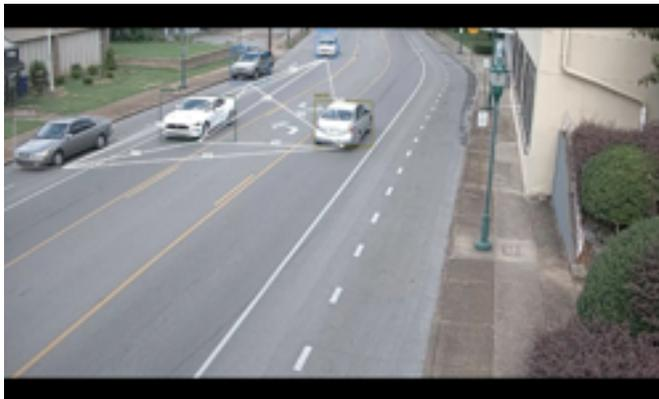
Real-time analysis of video data identifies situations where moving vehicles (and pedestrians) come too close to each other – known as “near miss” incidents. Object tracking on the MLK Smart Corridor gives us the ability to measure distances between objects in the camera’s field of view to discover the conditions that create near miss incidents. Our hope is that by learning more of what creates these incidents, we can mitigate them.
